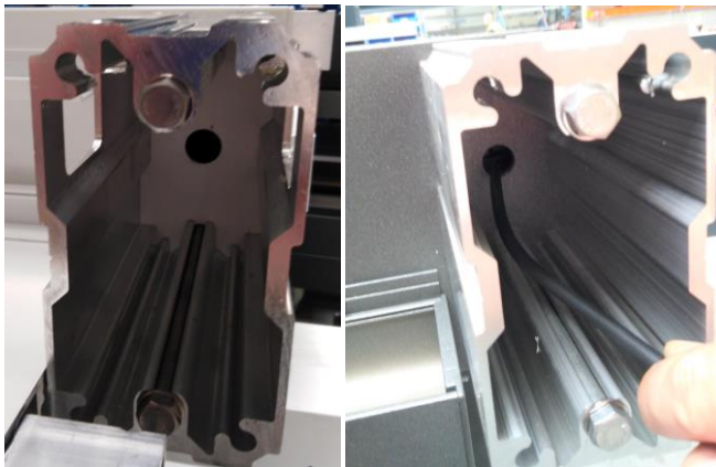
Fig. 8b Holes for wiring
